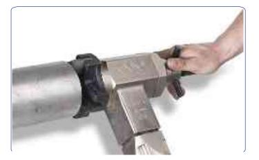
The Jaw system itself consists of 3 equilaterally positioned machined jaw segments, retained and locked on an inner, 'grooved' expansion shaft. These grooves keep the jaws held securely in position, unlike other systems that use a metal or rubber bands for jaw retention.
