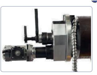
The Prep 20 has unrivalled power and stability, utlising a ratchet system for both jaw locking, and bevel feed.
