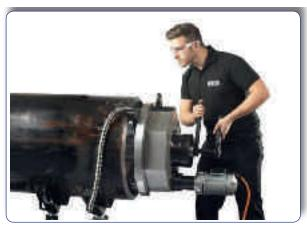
The PREP 24 has unrivalled power and stability, utilising a ratchet system for both jaw locking, and bevel feed.
